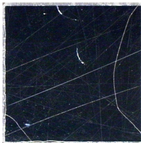
Fig. 2 4.0 by 4.0 mm die with two cracks
